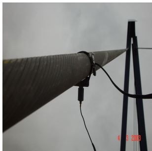
Figure: Damage detection on the Roberval bridge - Summer/Winter effect. Collaboration LCPC/KUL
